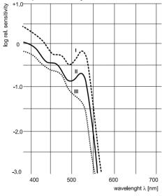
The values stated show the densities of 0.5 (I), 1,0 (II) and 1,5 (III) measured in reflection. The sensitivity is the reciprocal of the exposure in (mJ/m²) needed to produce the relevant densities.
